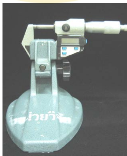
Fig. 4.6 Digital Micrometer, Mitutoyo No 293-421 N
