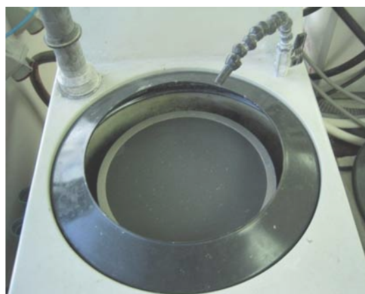
Fig.4.3 Rotary Pregrinder, Metaserv 2000, 300 cycle/min
