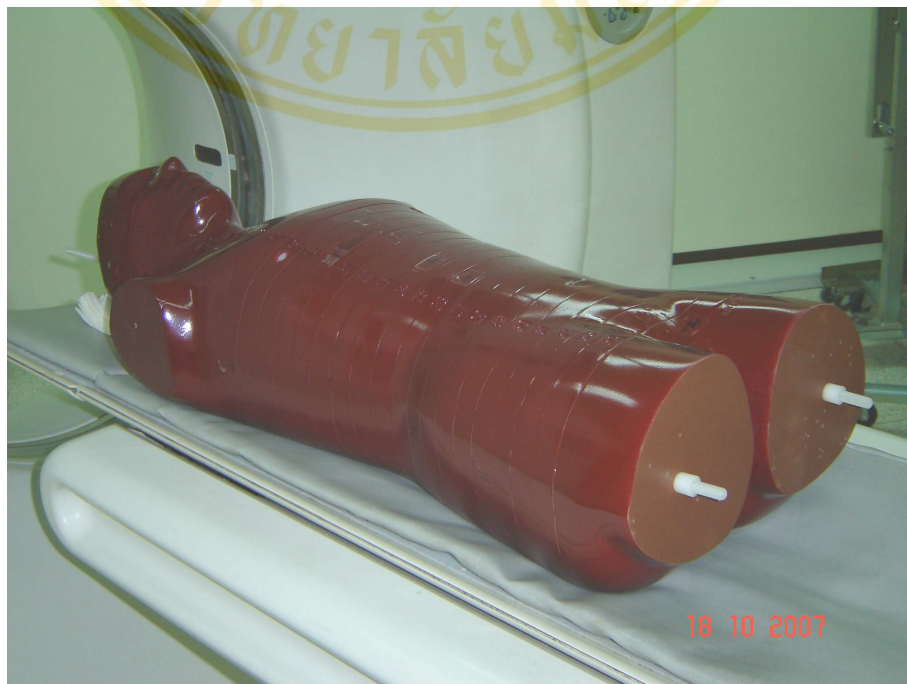
Figure 4.1.4 Male Alderson Rando phantom
