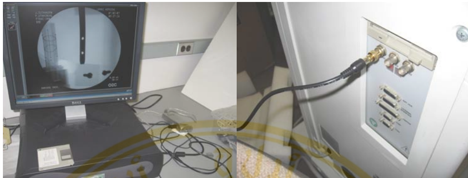
Figure 4.26 a) The TV encoder is connected to the PC monitor, which makes less time for saving the images from C-arm b) the TV encoder is connected to the C-arm.
