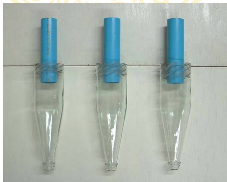
Figure E-2 Sauce bottle cyclones pattern I, II and III respectively
