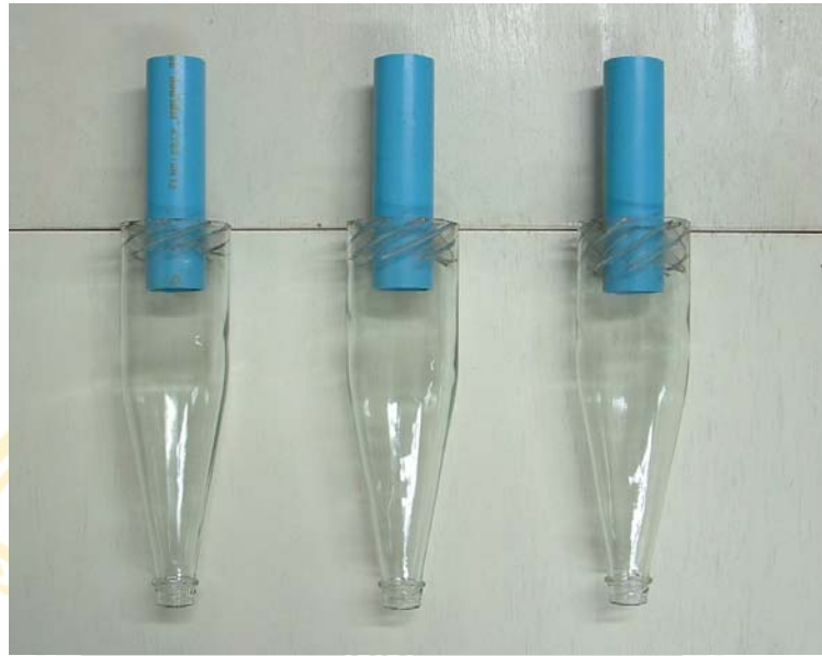
Figure E-3 Sauce bottle cyclones pattern IV, V and VI respectively
