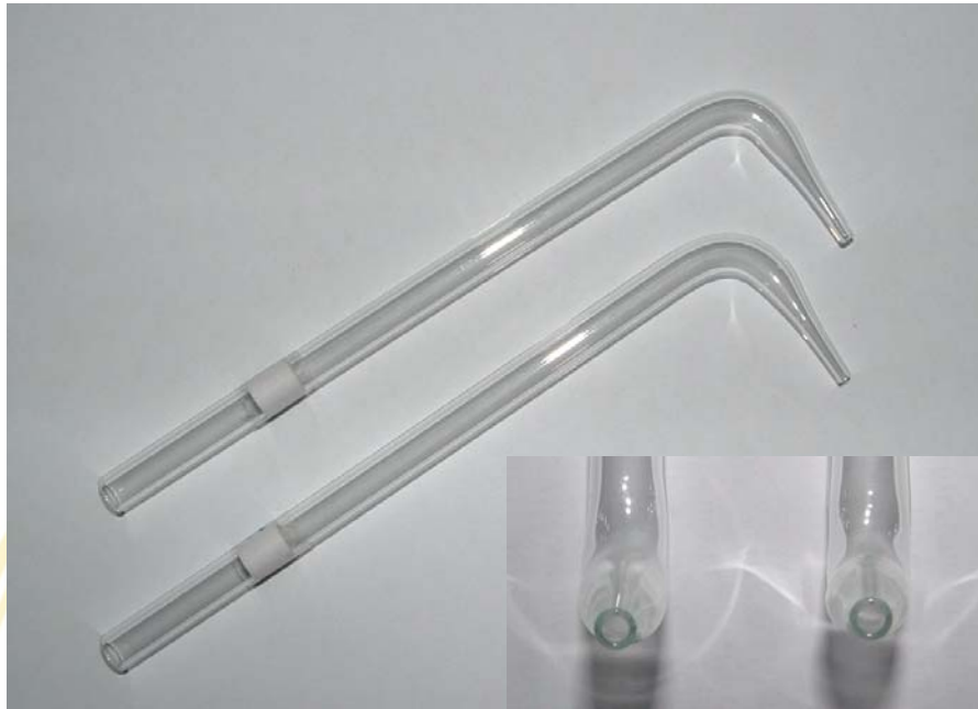
Figure F-3 The characteristics of glass sampling probes
