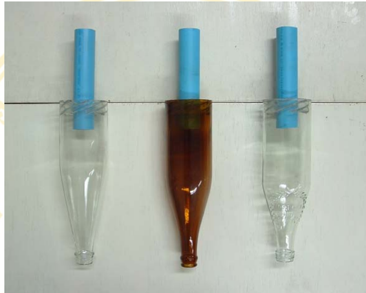
Figure E-1 Glass bottle cyclones which constructed from Sauce, Beer and Nectar bottles respectively
