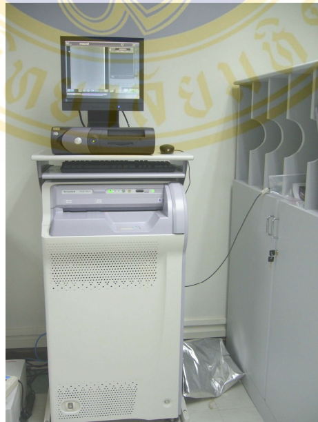
Figure 2 Fuji XG-1 Computed Radiography system
