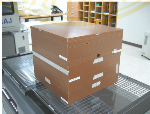
Figure 9. The solid water phantom (RMI) is made in square slab of 30 \times 30 \text{ cm}^2 with the thickness of 0.5, 1.0, 2.0 and 5.0 cm.
