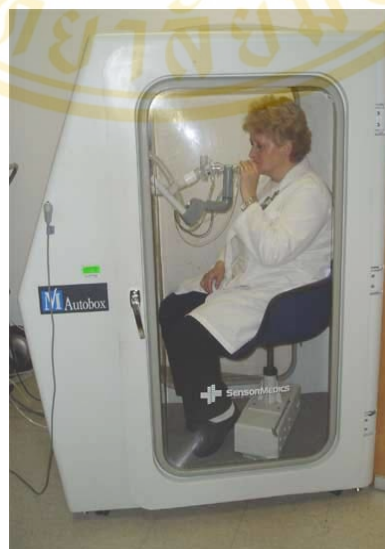
Figure 2.6 A plethymography “body-box” used to determine R_{aw} with multiple volume and pressure transducers mounted on the wall of this closed system make it possible to define compliance, flow, volume and resistance of airways.
