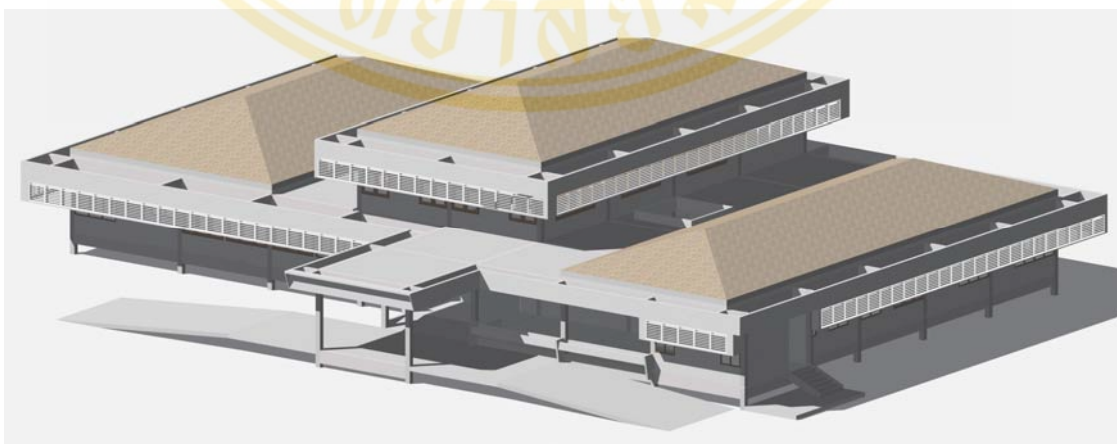
Figure 4.23 An isometric rendering of the Forth Prototype (The Second Prototype with shading devices)
