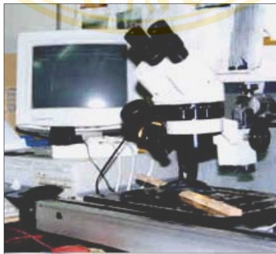
Figure 3-3 The moving stage and microscope interfaced with a computer
