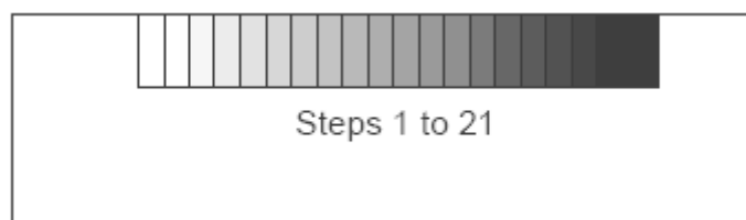
Figure 3: Representation of a Sensitometry Strip with 21 Steps of Measured Densities
