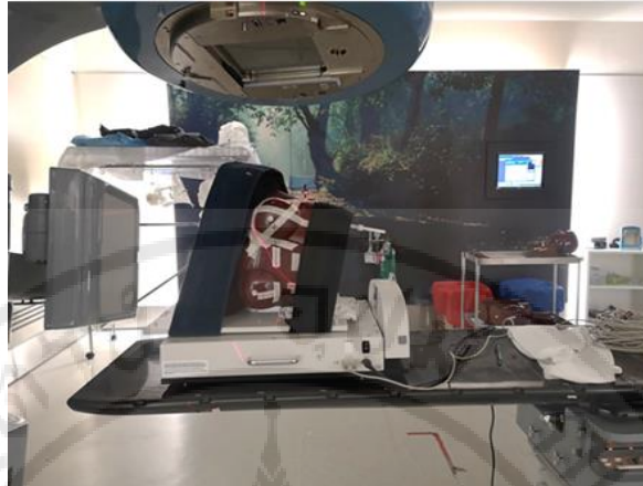
Figure 3.10 Setting the Rando phantom with MotionSim-4D/XY on LINAC.
