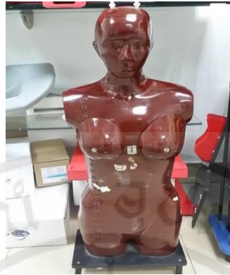
Figure 3.4 The Alderson Radiation Therapy Phantom [63].
