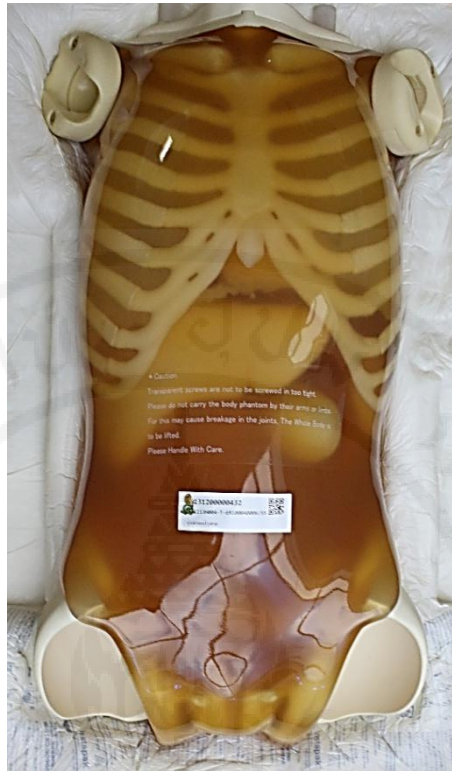
Figure 4.3 Anthropomorphic phantom (body phantom), thoracoabdominal part, embedded organs: lungs with vessels, mediasternal space, liver, kidney and pelvic girdle.
