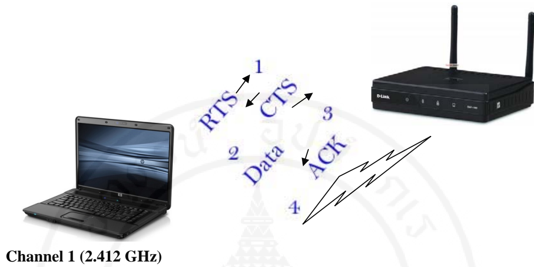
Figure 2.3 The operation of Wireless LAN protocols on Carrier Sense Multiple Access with Collision Detection (CSMA/CD).
