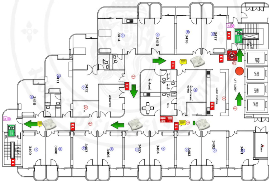
Figure 3.10 Diagram of the installed access points on the 12A-th floor of inpatient, Vibhavadi hospital.
