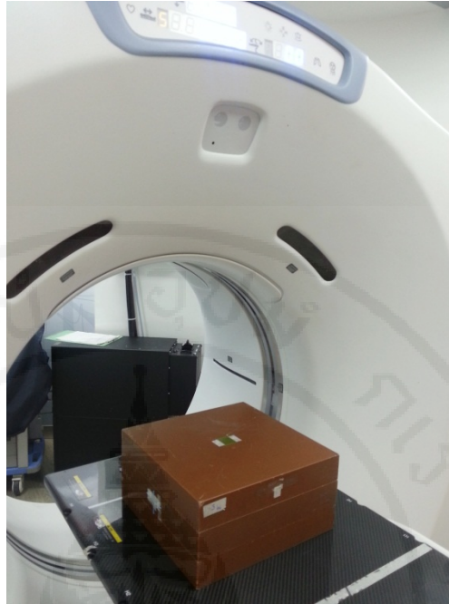
Figure 4.13. Setup of the solid water phantom with EBT2 film placed at the surface for CT scanning.
