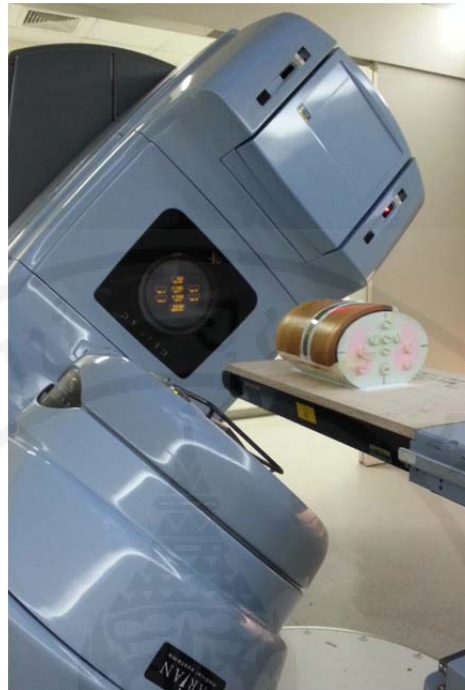
Figure 4.18. The measurement of tangential technique in lateral field with beam angle of 224.9 degree.
