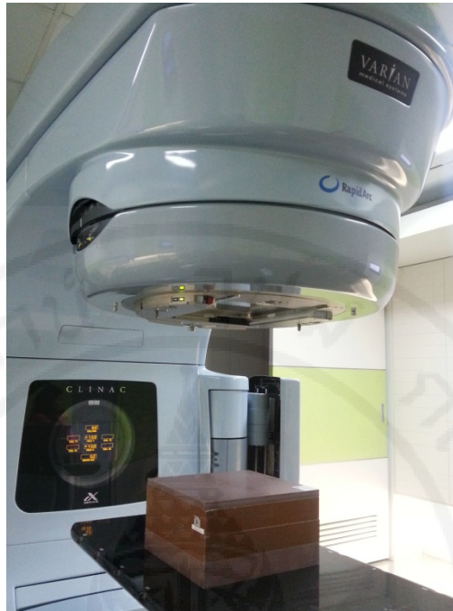
Figure 4.17. The measurement of direct angle at depth of 20 mm verification and field size of 10 \times 10 \text{ cm}^2 .
