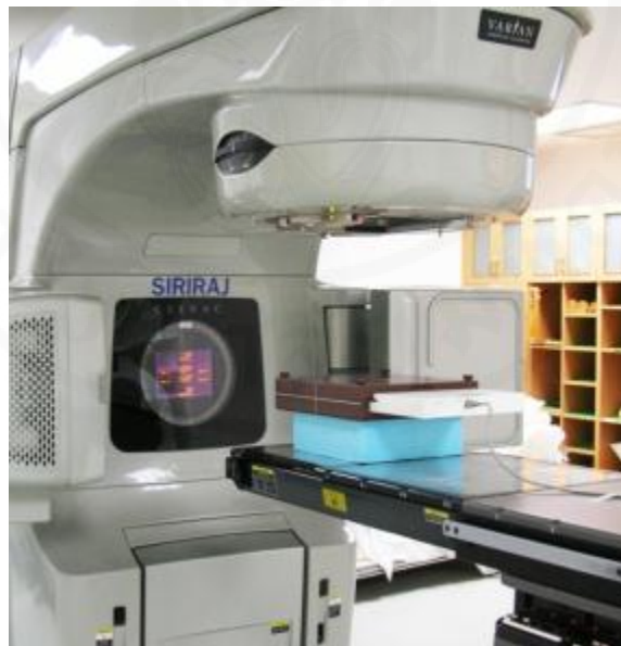
Figure 4.17 2D dose distribution IMRT verification using MapCHECK2™ and MapPHAN™
