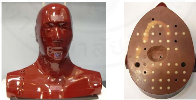
Figure 4.6 Anthropomorphic phantom: Anderson radiation therapy phantom (ART)
