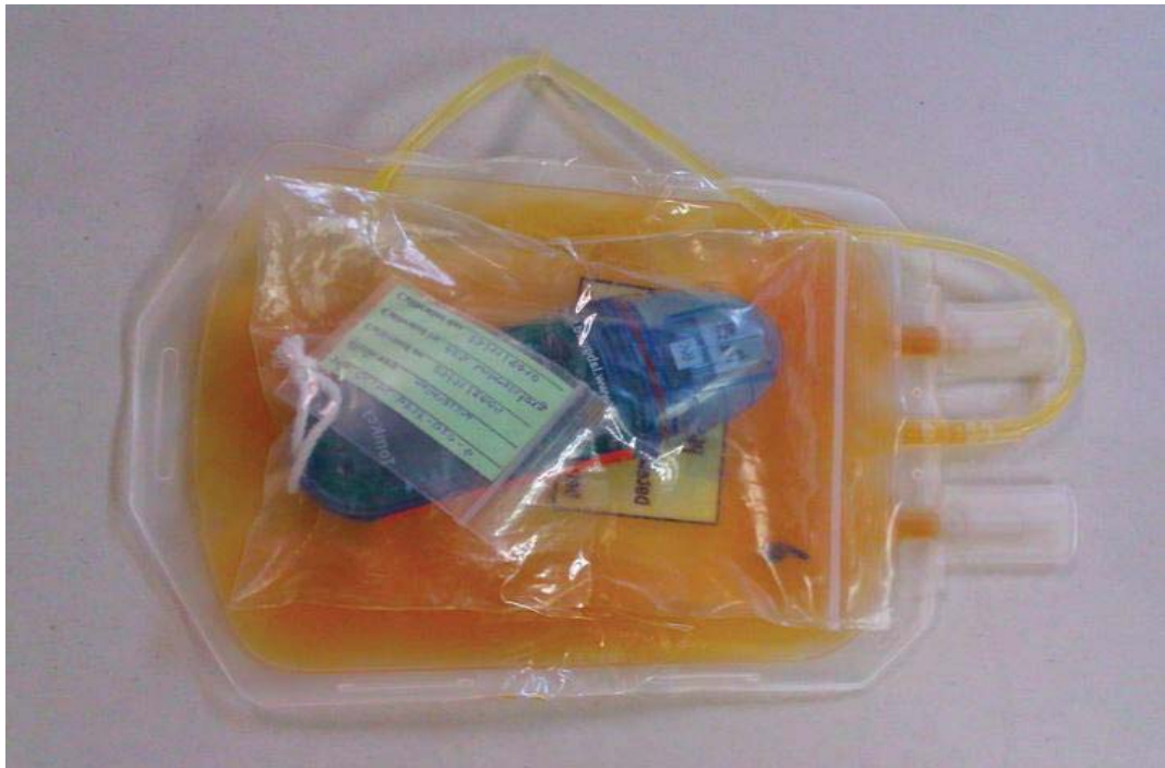
Figure 4.10 Tracking temperature using a data logger
