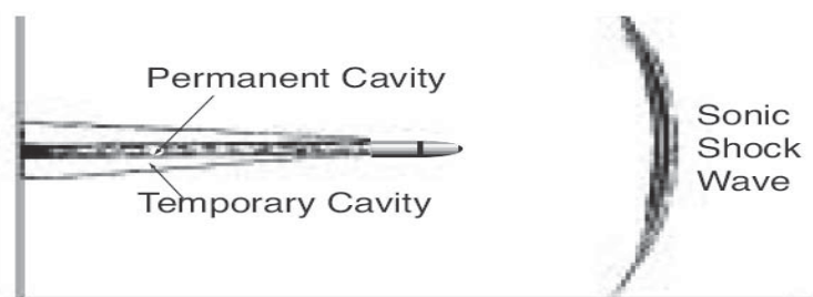
Figure 2.1: Projectile-tissue interaction, showing components of tissue injury.
