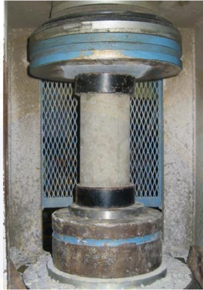
Figure 3.10 The Compressive Strength Test Setup
