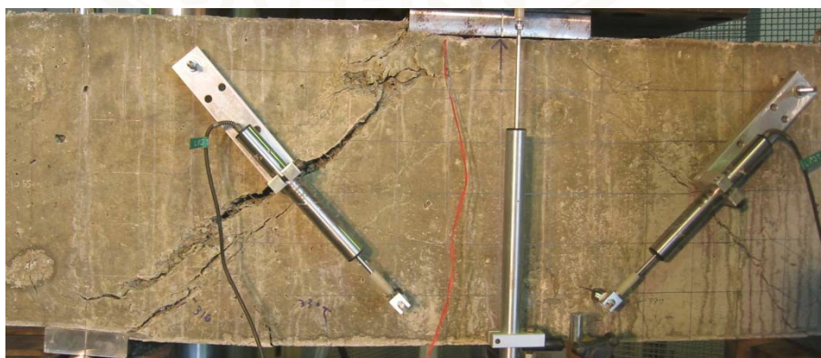
Figure C.35 Failure Mode for BF1.0-800
