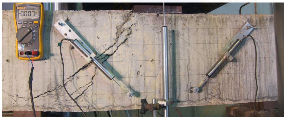
Figure C.34 Failure Mode for BF0.5-800
