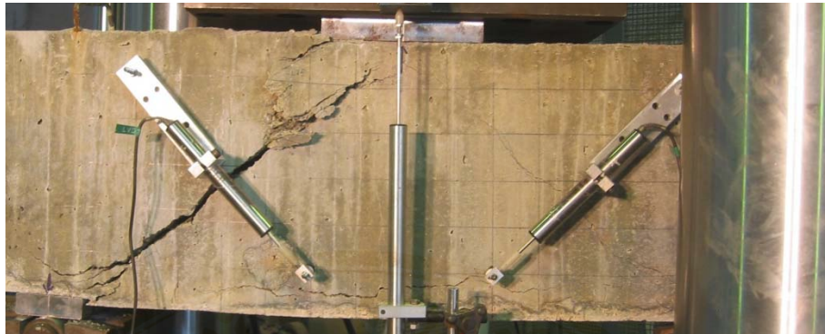
Figure C.33 Failure Mode for BF0.1-800
