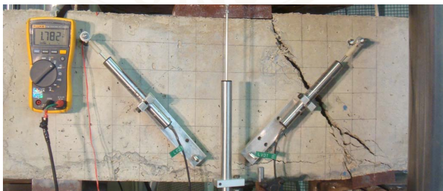
Figure C.38 Failure Mode for BPC-600
