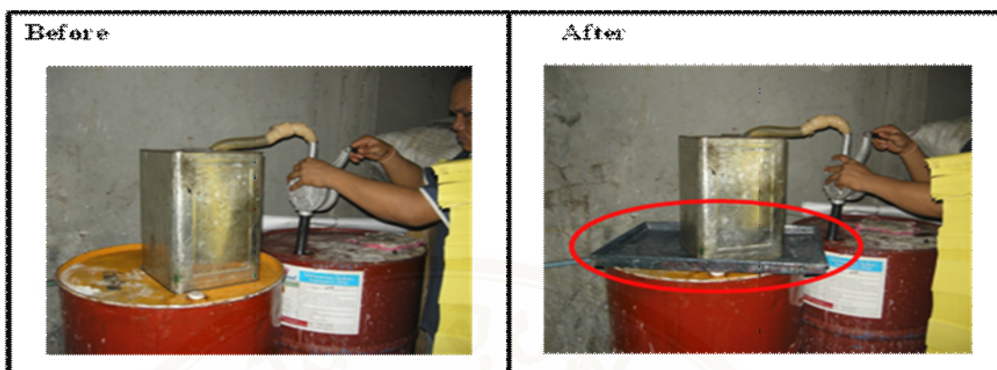
Figure 4.21 Secondary tray was placed below chemical container to trap the chemicals from chemical spills
