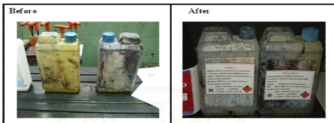
Figure 4.26 Chemical container that transfer from large containers was labeled
