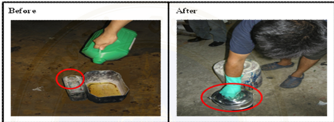
Figure 4.45 After finished usage, lid of chemical container was tightly closed to protect chemical spreads
