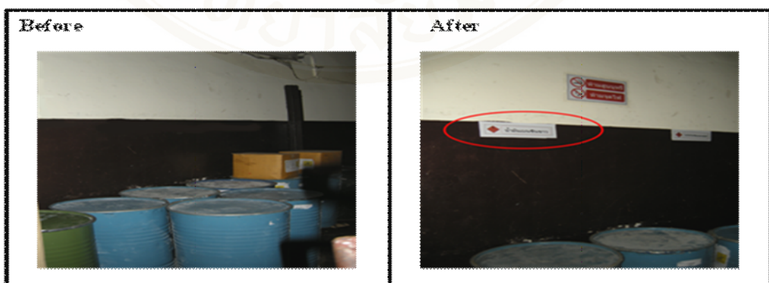
Figure 4.9 Warning sign or chemical label for hazardous chemicals were marked in the chemical storage facility
