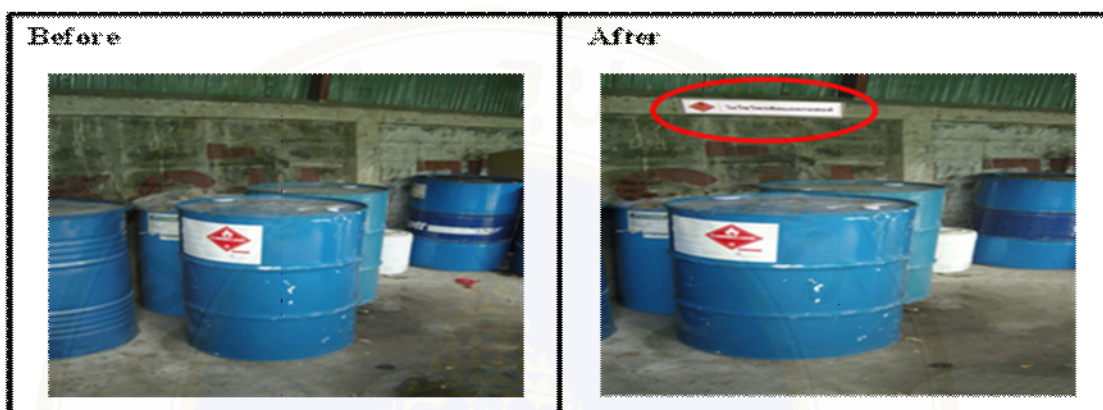
Figure 4.33 Warning sign or chemical label for hazardous chemicals were marked in the chemical storage facility
