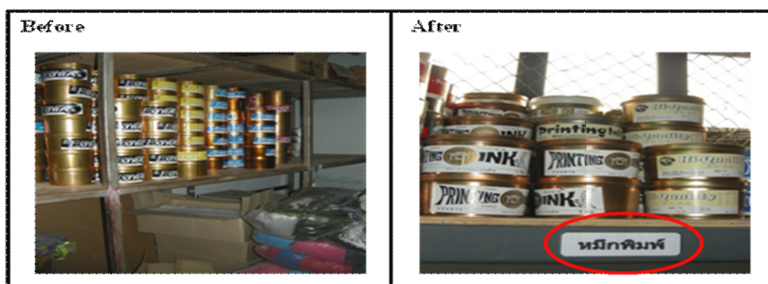
Figure 4.32 Chemical storage shelves have the chemical label
