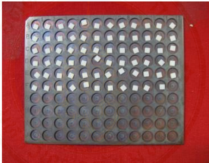
Figure 4.3 The chips of thermoluminescent dosimeters (TLD-100H).
