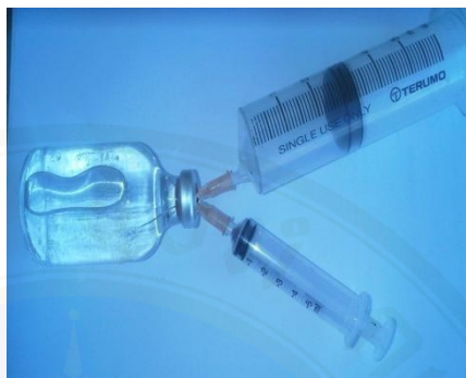
Figure 3.5 The water displacement to obtain mixture of gas
