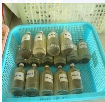
Figure 3.4 The biochemical hydrogen potential test
