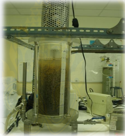
Figure A-1. Cassava ethanol spent wash operated under dark fermentation by Semi – Completely Mixed Reactor
