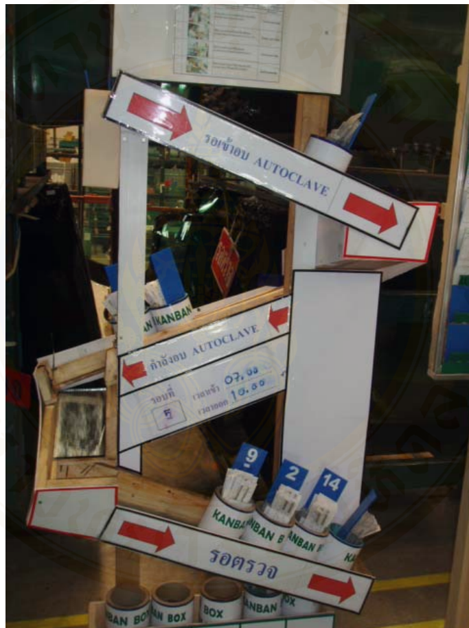
Figure 4.38 Progressive Post in Autoclave division
