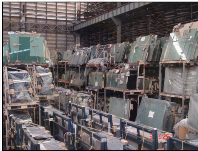
Figure 4.2 Storage layout for glass material before TPS
