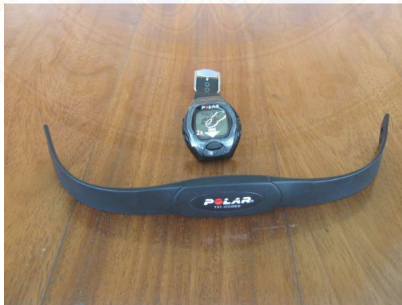
Figure 6 Telemetry heart rate Monitor (Polar Accurex Plus, Finland)
