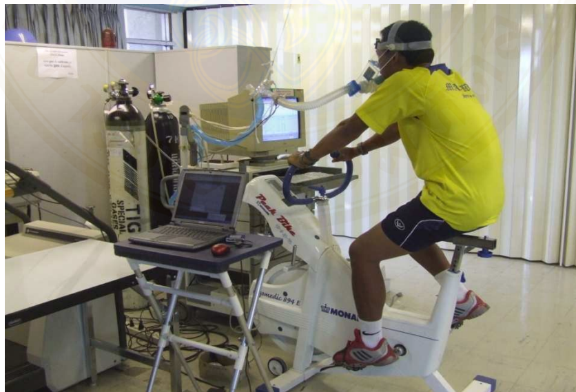
Figure 4 Metabolic test System (Gas analyzer Seensormedics Vmax 229, USA)
