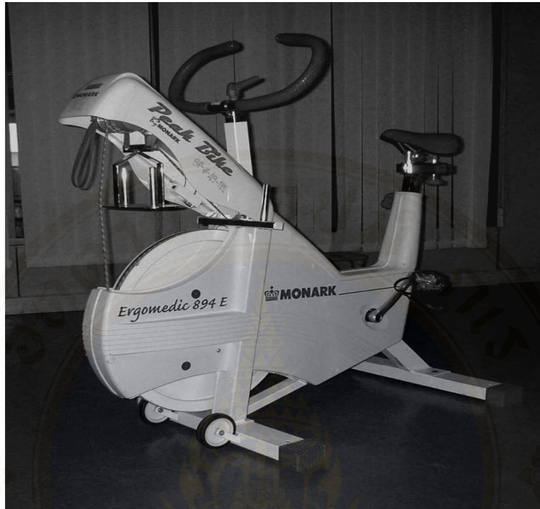
Figure 5 Cycle ergometer (Monark 894E, Sweden) with calibrated weight.
