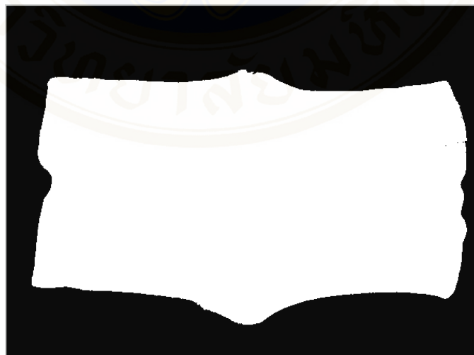
Figure 3.6 Example of binary Ribbed Smoked Sheet from Otsu's Method
