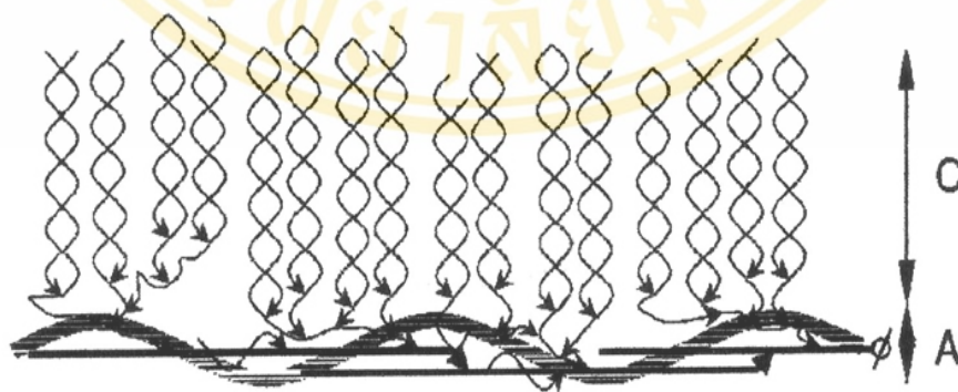
Figure 4 The two-directional backbone model in a normal starch, where the amylose (thick wave-line) is found together with the amorphous chains of amylopectin (A: Amorphous region; C: Crystalline region)(Bertoft, 2004)
